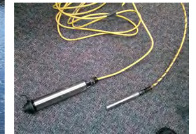
Figure 23: Pressure Transducer Used to Measure Water Level in Streams
