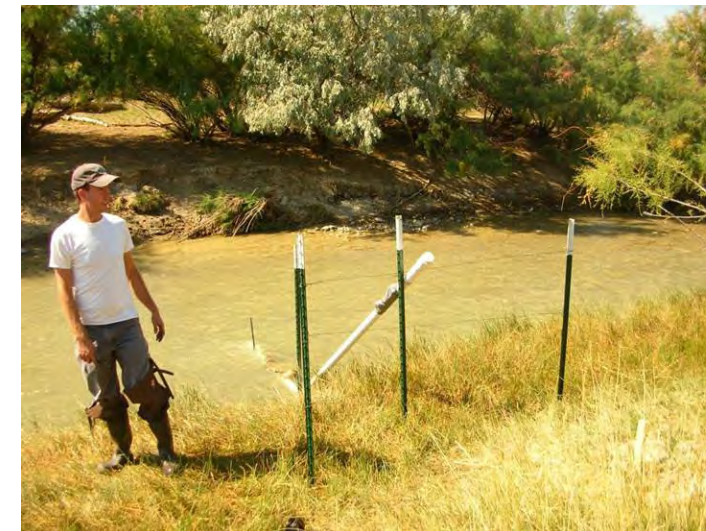
Figure 24: Temporary Stream Gauge
